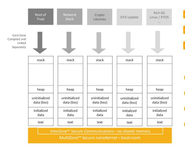
Multiple equally secure zones for programs, data, i/o Hardware-enforced Software-defined Policy-driven RWX
